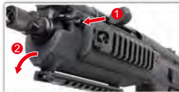
1. Pull the handguard locking pin out. 2. Disassemble the handguard.
