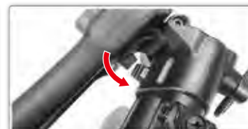
Hook the stock onto the receiver.
